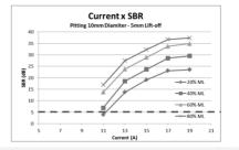
SBR evaluation for a 10 mm diameter pitting in different magnetization levels
