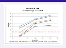
SBR evaluation for different crack depth using different magnetization levels (by electrical current application).
