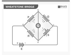
Here if, P/R = Q/S or P/Q = R/S, then, we can simply remove G. Now, P & Q are in series and R & S are in series, and the combination of the two are in parallel
