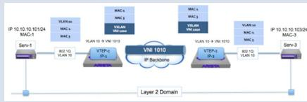
The ingressing VTEP will map the VLAN to the VNI and encapsulate the packet with a VXLAN header with the VNI destined to the VTEP IP of the remote host found in "show vxlan address-table". Once the remote VTEP receives this packet, it decapsulates the packet and does the reverse VNI to VLAN mapping. The packet then switches per normal L2 (mac address table lookup).
