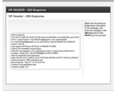
Via headers are inserted by servers into requests to detect loops and to allow responses to find their way back to the client VIA the server
