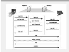
100 trying - progress of the call setup 180 ringing - when the destination starts ringing 200 Ok - message is sent on device pick-up which is relayed and followed by an acknowledgement.
