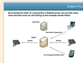
The proxy can receive all respond from possible destinations and send back only the appropriate 200 response without maintaining state an agent would have sent 3 invites and maybe received the errors before the live agent could respond, resulting in call setup failure.
