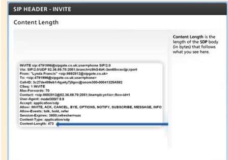
The header indicates the method type. eg INVITE, the SIP URI of the target UA and SIP version 2.0
