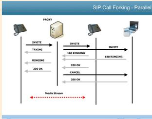
With call forking in 'parallel mode', the SIP proxy receiving the INVITE will discover via the location server that you have two current locations. It will send an INVITE to both locations at the same time
