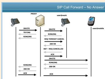
Proxy sends an INVITE to a device which rings and responds back to the proxy. After a configurable timer has expired on the proxy, the proxy sends a cancel to the device that responds and then the proxy sends an INVITE to the call forward number the proxy has for the user.
