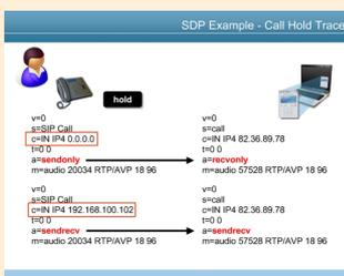
To put a call on hold, the holding device sends connection details of an IP address of 0.0.0.0 and an audio setting of **sendonly** which the receiving device responds back with **recvonly**. Press hold to re-establish the media stream resends the appropriate connection IP address along with the **sendrcv** attribute. The receiving device responds with **sendrcv** and two way audio is reestablished.
