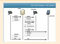
Proxy sends an INVITE to a device which rings and responds back to the proxy. After a configurable timer has expired on the proxy, the proxy sends a cancel to the device that responds and then the proxy sends an INVITE to the call forward number the proxy has for the
