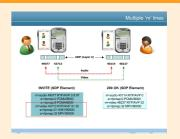
multiple 'm' lines - The SDP INVITE element shows the m=auio element for the voice including port info and the m=video element details the port and other requirements for the video. When the calling received the 200 OK to both elements the voice and video channels are set up.
