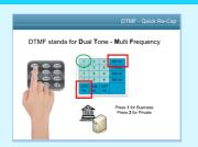
DTMF - dual tone - multi frequency When you press the buttons on a telephone keypad, a connection is made that generates two tone at a time, a row tone and a column tone.
