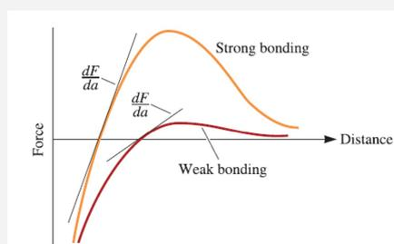
Stiffness of a material is related to the slope of the F vs atomic separation curve (r). The stiffness (dF/da) of the material is known as the **Young's modulus, E**.
