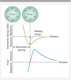
Equilibrium separation occurs when the total energy is minimized and also when the net force is zero.
