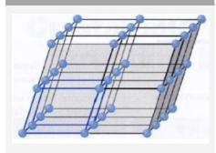
A collection of points arranged on a periodic pattern so that the surroundings of each lattice point are identical.
