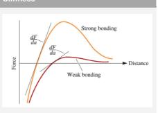
Stiffness of a material is related to the slope of the F vs atomic separation curve (r). The stiffness (dF/da) of the material is known as the **Young's modulus, E.**
