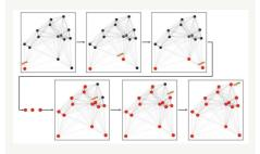
In this algorithm, an artificial ant must simulate a path starting at a specific point. It moves node by node, choosing based on the pheromones of each path.
