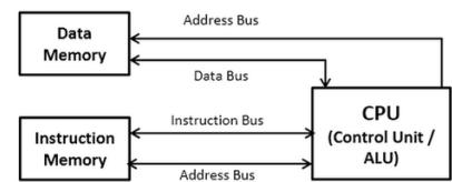
In the **Harvard Architecture**, data and instructions are stored separately and accessed via separate buses. The Harvard Architecture is generally used by **RISC** processors.
