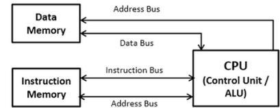
In the **Harvard Architecture**, data and instructions are stored separately and accessed via separate buses. The Harvard Architecture is generally used by **RISC** processors.
