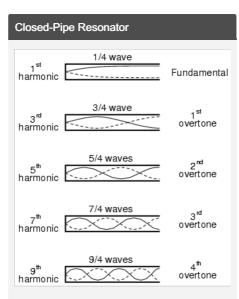
Closed-Pipe Resonator: tube is closed at one end and open at another
