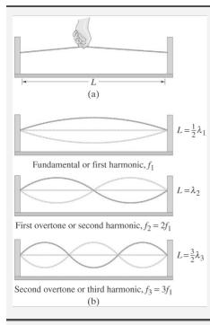
Stringed Resonator: a resonating instrument that is fixed at both ends
