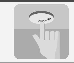
Test smoke alarms at least once a month using the test button.
