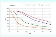
Figure 3: If an application requires 80 oz.-in. of torque up to 20 rps, the motor should use a 48-V power supply, as shown by the graph. The process of sizing an application involves calculating the required torque and speed range necessary to move the load. For example, if the application needed 80 oz.-in. of torque up to 10 revolutions/second (rps), this motor could use a 24-V power supply (see Figure 2)
