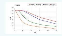
A PWM driver will increase the voltage applied to the motor to keep the current and torque constant. At some speed, the power supply will not have enough voltage, and the motor current will begin to fall. The torque drops with the current. If using a higher voltage power supply, the dynamic torque remains flat to a higher speed (see Figure 1).
