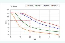
If we need to go farther and faster, one might accelerate to 80 oz.-in. at 20 rps. The motor would require a 48-V power supply (see Figure 3)
