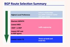
BGP uses both policy and shortest path based routing.
