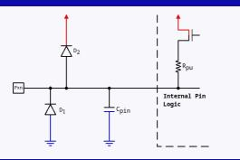
All pins have diodes to protect against undervoltage (D1) and overvoltage (D2).
